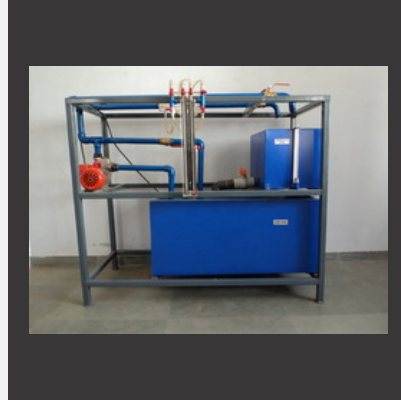
Venturimeter & Orificemeter Test Rig
